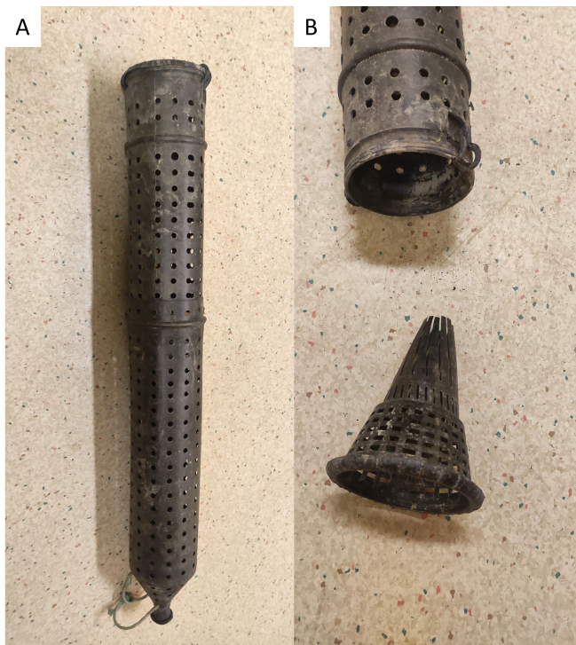
Figure 2. Self-designed habitat trap in the form of perforated PVC pipe (A); funnel-shaped ends allowing the organisms to enter, but not to escape (B).
